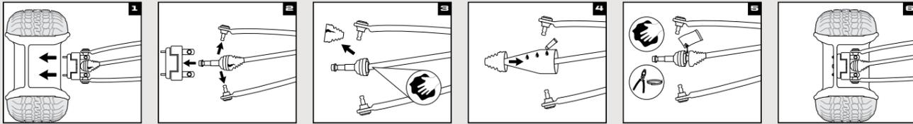
1. Remove wheel and axle nut.
